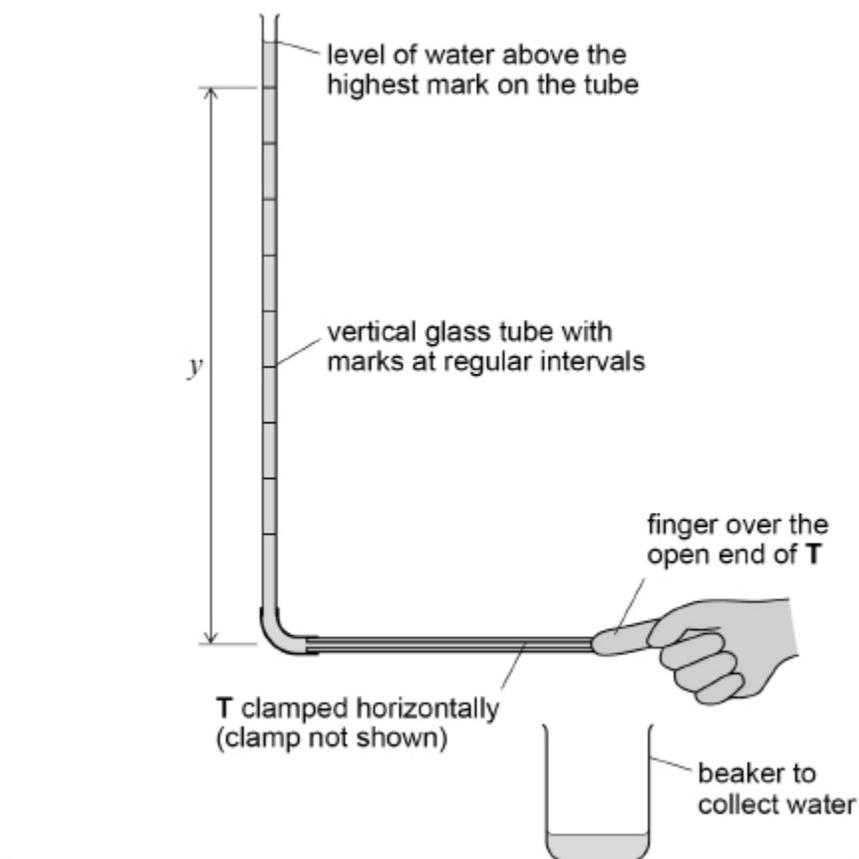
**T** is opened and water flows into a beaker. When the water level falls to the highest mark on the tube, she starts a stopwatch. She records the time  $t$  for the water to reach each of the other marks.
